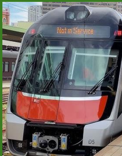
Figure 5: An intercity train with a multifunction coupler. Note the electrical heads on either side of the mechanical and pneumatic connections
