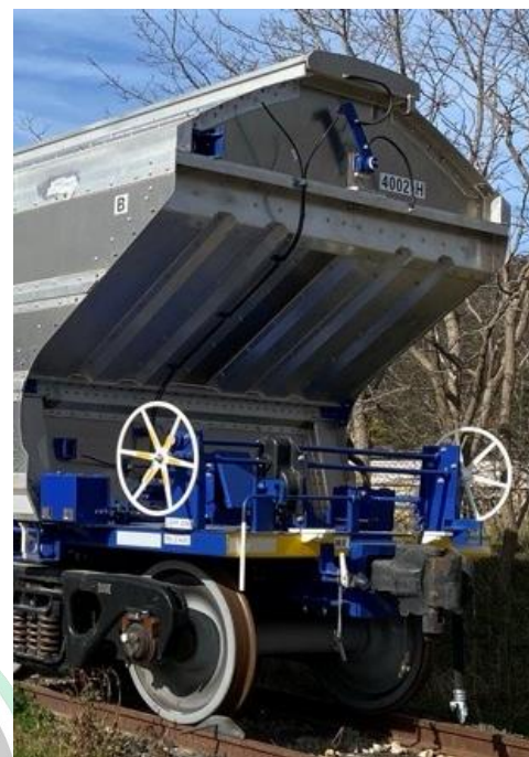
Figure 3: a typical freight wagon with a knuckle type automatic coupler, brake hoses and handbrake wheels. Note also the chocks fitted under the lead bogie.
