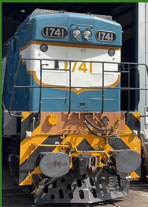
Figure 2: a typical diesel electric locomotive with automatic knuckle coupler, various brake related hoses and multiple unit electrical coupling receptacle. Of note, this locomotive is also fitted with side buffers for heritage operations.
