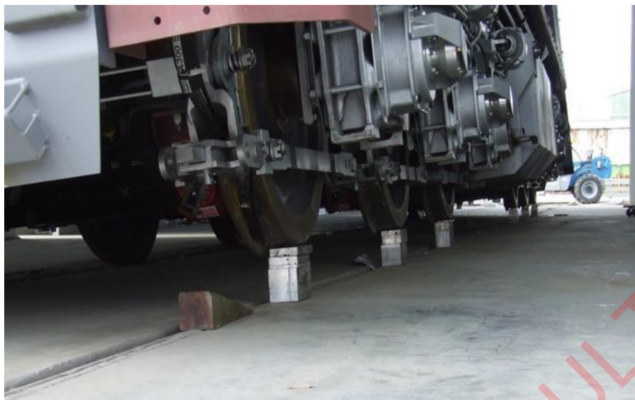
Appendix Figure C-1 Static kinematic test setup (wheels packed to maximum test cant)
